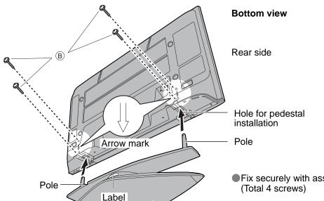
Fix securely with assembly screws B.
